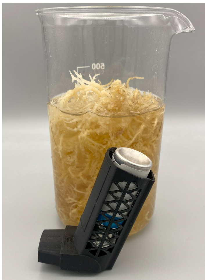
FIGURE 3. Seaweed-based biomaterial used to 3D print an inhaler prototype
